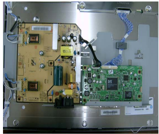
3. Separate cable Main Board and Separate screw between Shield PCB and Bracket PCB.(2 point)
